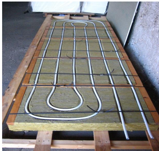
Fig.8. Prototype of thermal insulation panel ATP - supporting frame - mineral wool, dimensions 2000 x 1000 x 100 mm (heat transfer medium WATER) [author - Kalús, D.]
