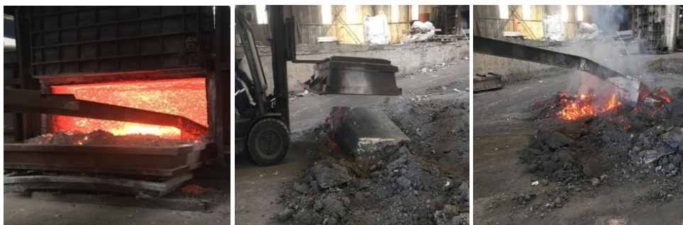
Figure 1. Stage of dross extraction and processing
