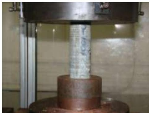
**Fig.6.** A sample under UCS test
