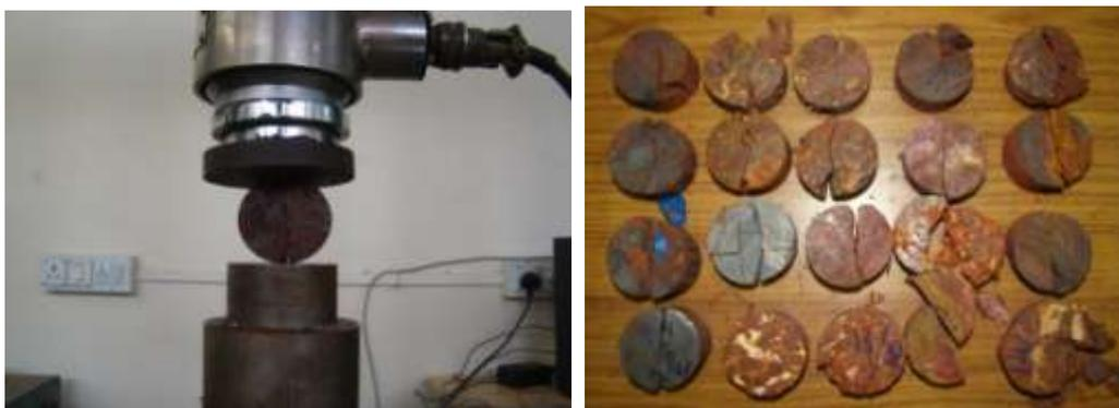
Fig. 14 Samples under Uniaxial Tensile Strength test (Brazilian test)
