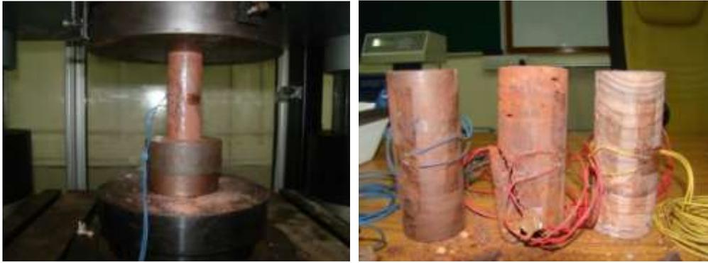
Fig.7. Samples under UCS test with lateral strain gauge
