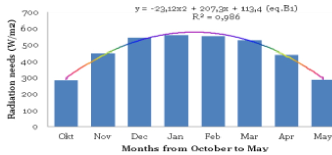
Fig. 22. Average values of solar radiation needs in W/m 2 , from October to May, in climatic zone B.
