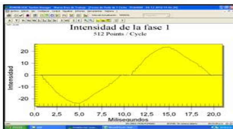
Fig. 5: Screen of the software POWERLOGIC System Manager SMS 121 with the resulting waveform obtained in one measure
