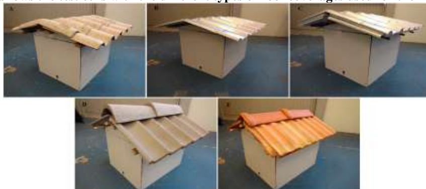
Figure 3. Test cells with assembled roofs (A) Fiber-cement tiles; (B) Aluzinco tiles; (C) "Sandwich" aluzinco tiles; (D) Concrete tiles; (E) Clay tiles.
