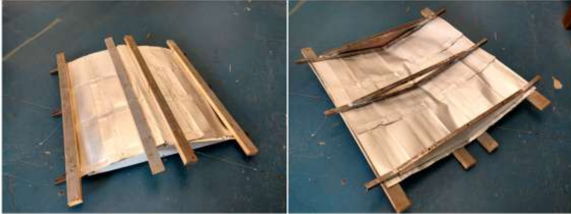
Figure 5. Roof structure with double-layer blanket.
