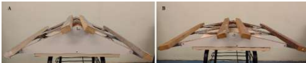
Figure 1. Roof structures (A) Roof structure for clay and concrete tiles; (B) Roof structure for fiber-cement, aluzinco and "sandwich" aluzinco tiles.
