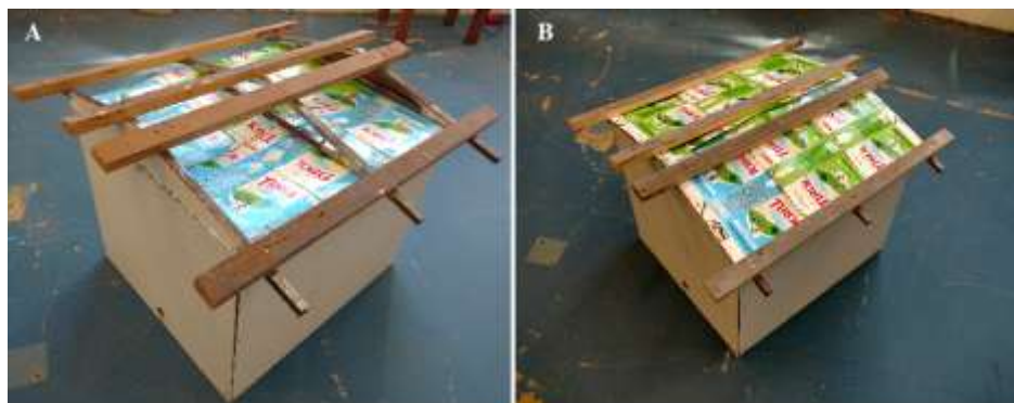
Figure 2. Blankets installed in test cells (A) Blanket as lining; (B) Blanket as roof undercoverage.
