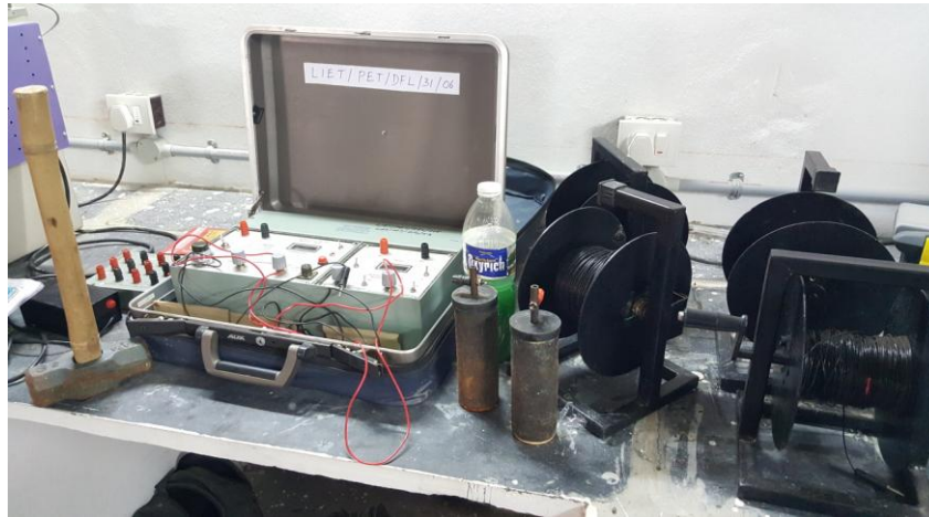
Fig.2 Apparatus of spontaneous potential of electrical resistivity
