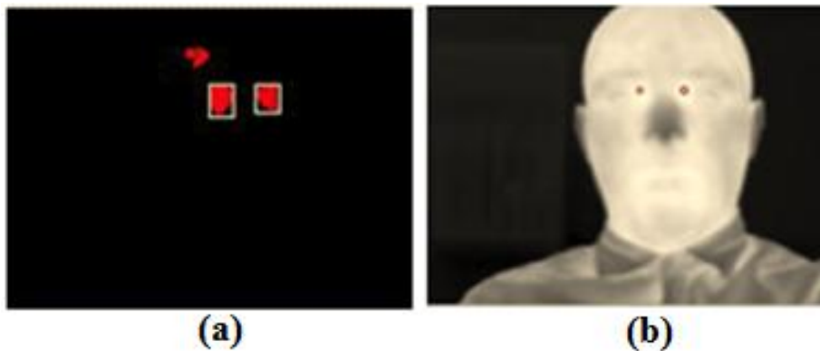
Figure 0-3: (a) Detection of eyes' corners in presence of more than two objects and (b) eye corners mapped onto image.
