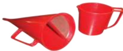
Fig.2, Marsh funnel are used to measure fluid viscosity.
