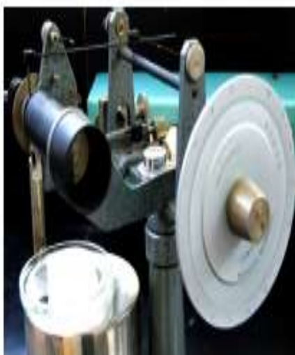
Fig.1, Tensiometer used for testing surface tension and IFT
