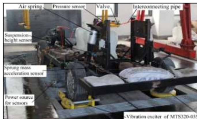
Fig 2.1: Test Bench of Interconnected Air Suspension System
