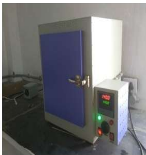
Figure 3: Copper strip apparatus
