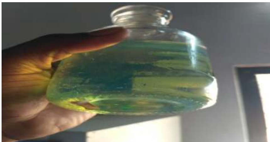
SFigure 5:- Copper strip in diesel
