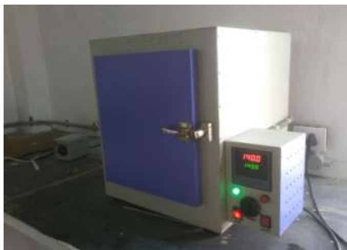
Fig.1 Copper strip corrosion apparatus
