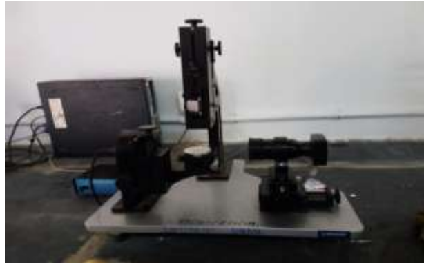
Figure. 6 Setup to determine drop image
