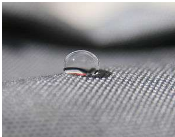
Figure.1 Cloth, treated to be hydrophobic, shows a high contact angle
