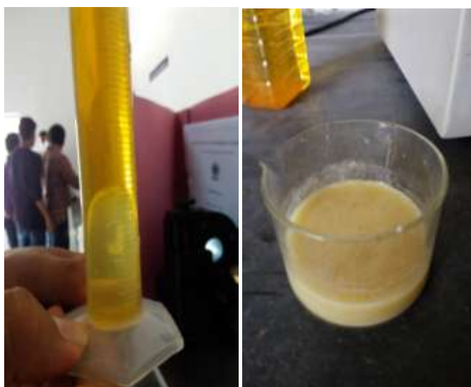
Figure. 5 Preparation of oil water mixture samples
