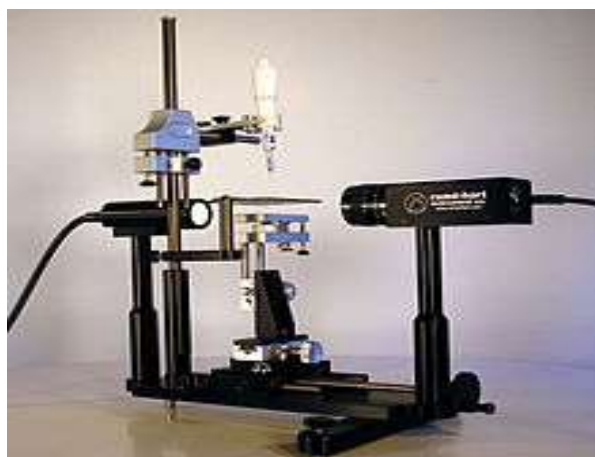
Figure. 4 Goniometer for contact angle analysis
