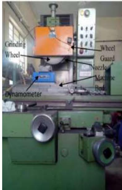
Fig.1 Surface Grinding M/c Setup
