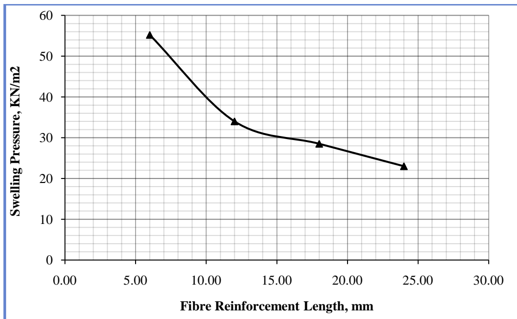
Figure.4.2: Improvement in Strength Characteristics of Expansive Soil-Fly Ash Mix in terms of Swelling Pressure with Different Length of Randomly Distributed HT Nylon-66 Fibres
