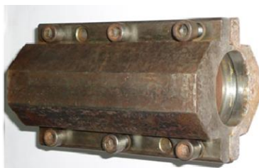
Two parts of the container assembled with bolts
