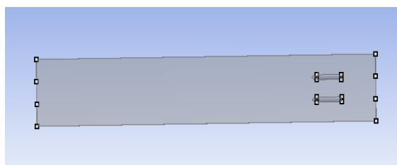
Fig.6 Top view of car with vortex generator kept straight to the flow field
