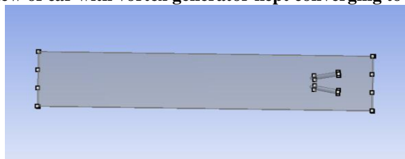
Fig.8 Top view of car with vortex generator kept diverging to the flow field
