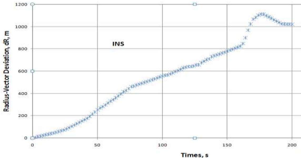
Fig. 9. Estimation error the radius vector
