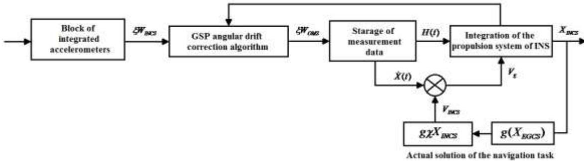
Fig. 4. A functional circuit for INS using GSP
