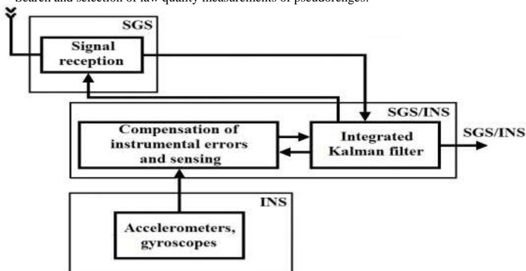
Fig. 1. Ultra-tightly coupled system [19]
