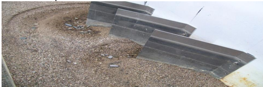
Figure 3. Picture of scoured bed surface at the equilibrium state
