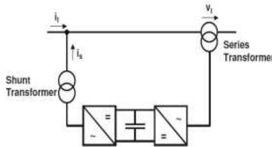
**Fig.2.**Principle configuration of an UPFC
