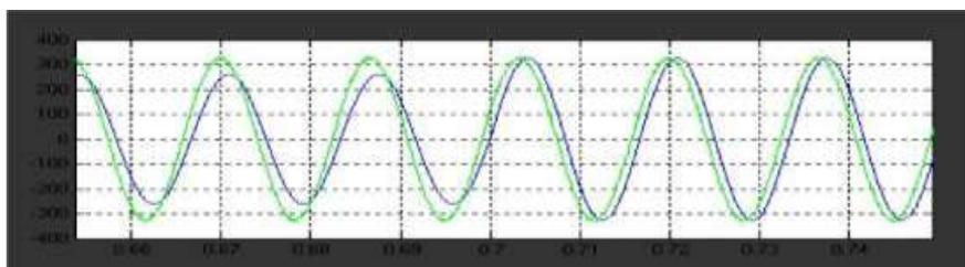
(i) Enlarged power angle  $\delta$  during voltage sag condition.
