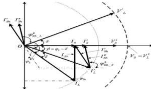
**Fig. 7.** Current-based phasor representation of the proposed UPQC-S approach under voltage sag condition.
