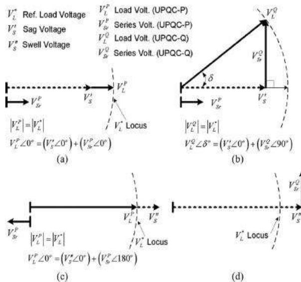
Fig. 4 Voltage sag and swell compensation using UPQC-P and UPQC-Q: phasor representation. (a) Voltage Sag (UPQC-P). (b) Voltage Sag (UPQC-Q). (c) Voltage Swell (UPQC-P). (d) Voltage Swell (UPQC-Q).
