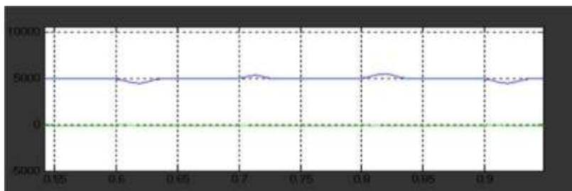
e) Enlarged power angle  $\delta$  relation between supply and load voltages during steady-state condition.
