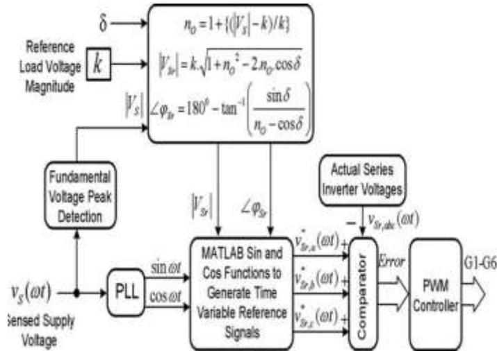
Fig. 11 Reference voltage signal generation for the series inverter of the Proposed UPQC-S approach.
