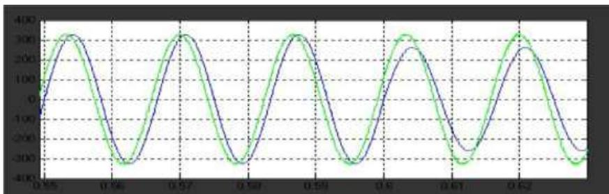
(h) Shunt inverter injected current
