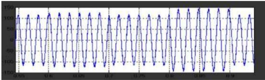
(c) Series inverter injected voltage
