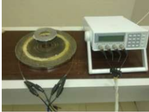
Fig.4. Experimental investigation of HTSC coil inductance with magnetic screen below the coil
