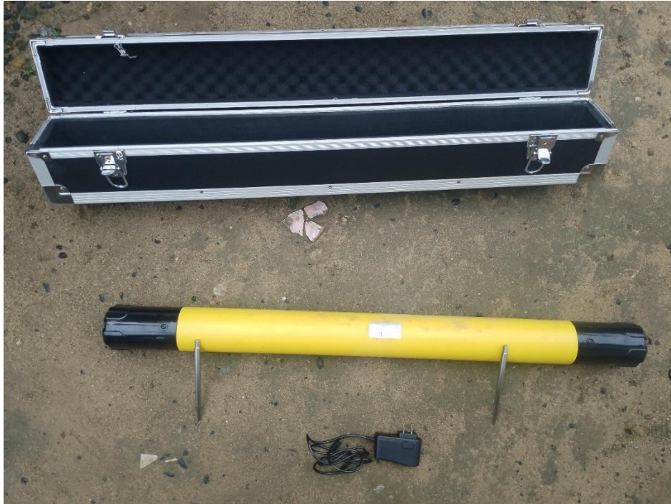
Figure 2: A digital Terrameter for Groundwater Exploration.
