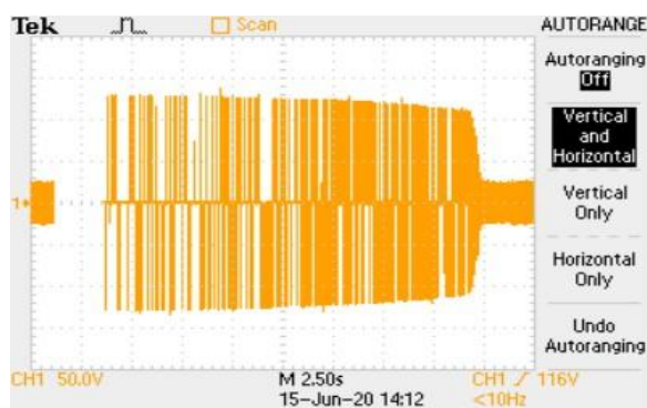
Fig -7: Response of BLDC Motor at steady state condition
