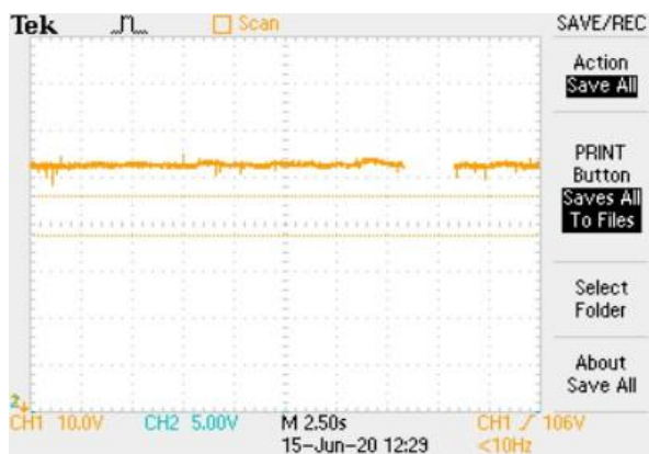
Fig -6: Response of PV Array at steady state condition
