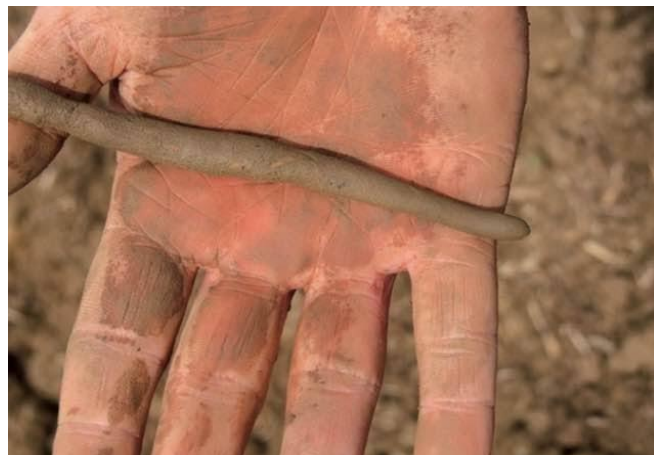
Fig.3 Plastic limit testing
