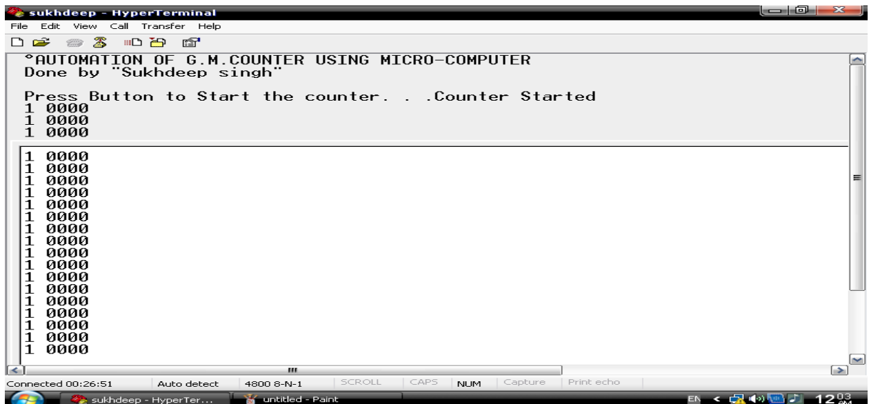
Figure 2:- Readings sent serially to the computer using HyperTerminal
